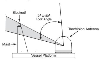
Figure 5: Antenna Dimensions
